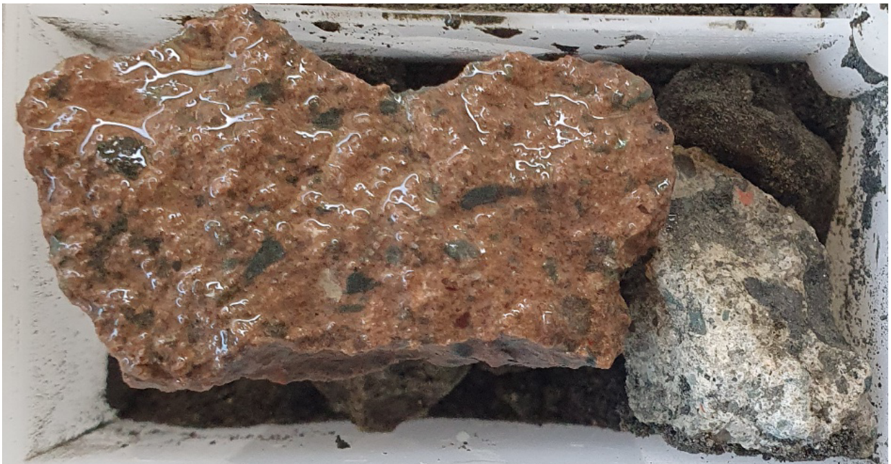
Figure 3: No mineral occurrence is being reported or claimed. These breccia chips at the base of hole NBG011 simply displays Quartz K-Spar porphyry rock fragments (the wet fragment is ~15mm long).
