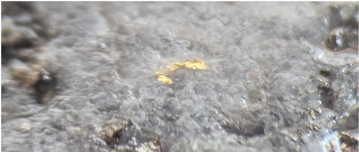
Figure 2. Visible gold in drill core from diamond drill-hole 25XCDD002 at 150.05m down-hole, the second instance of visible gold at the Martin Prospect. Field of view width 5mm, refer Table 1 and Figure 3 for additional information.
