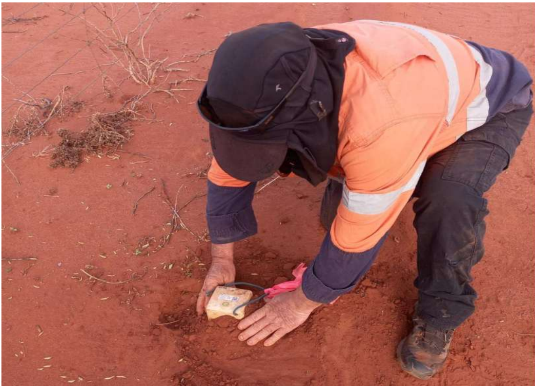
Image 1. Passive seismic survey in progress at the Yanrey Uranium Project
