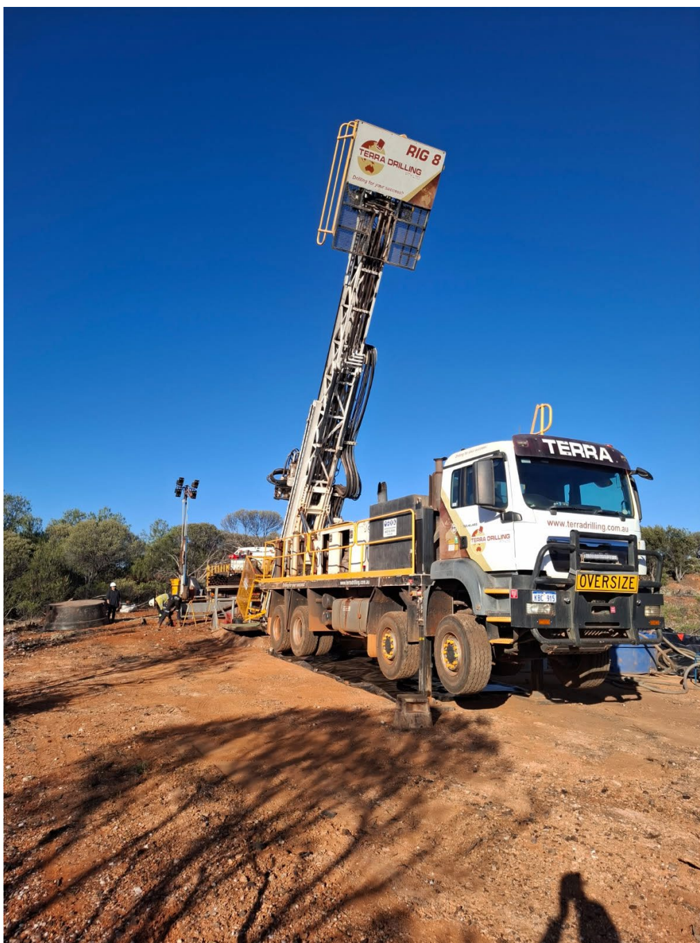
Above: Diamond drill rig on site.
