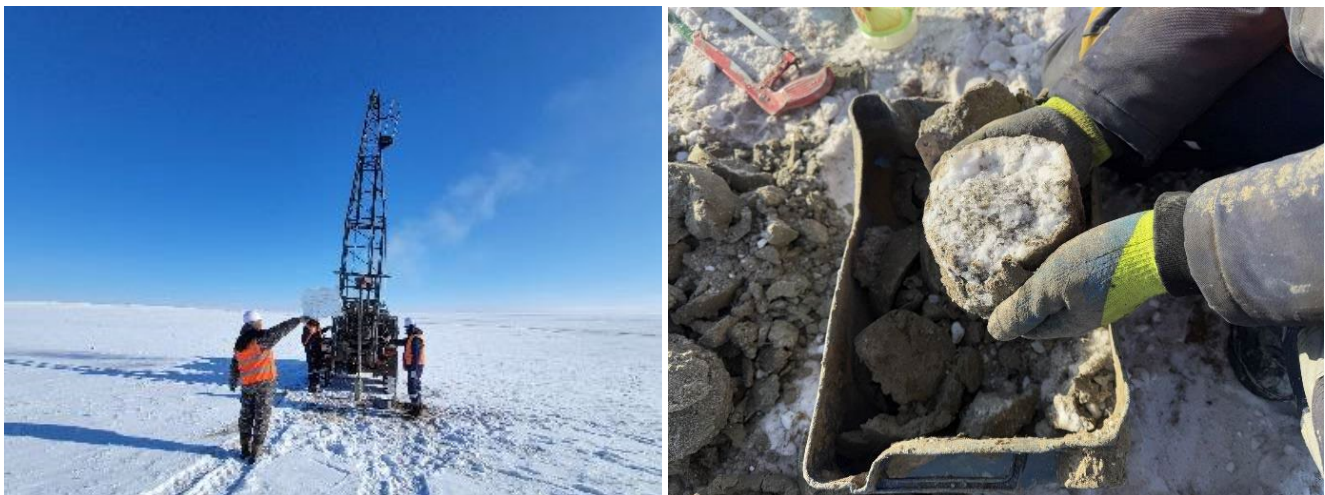
Geotechnical survey drilling and sample collection at Ovoot in January 2025
