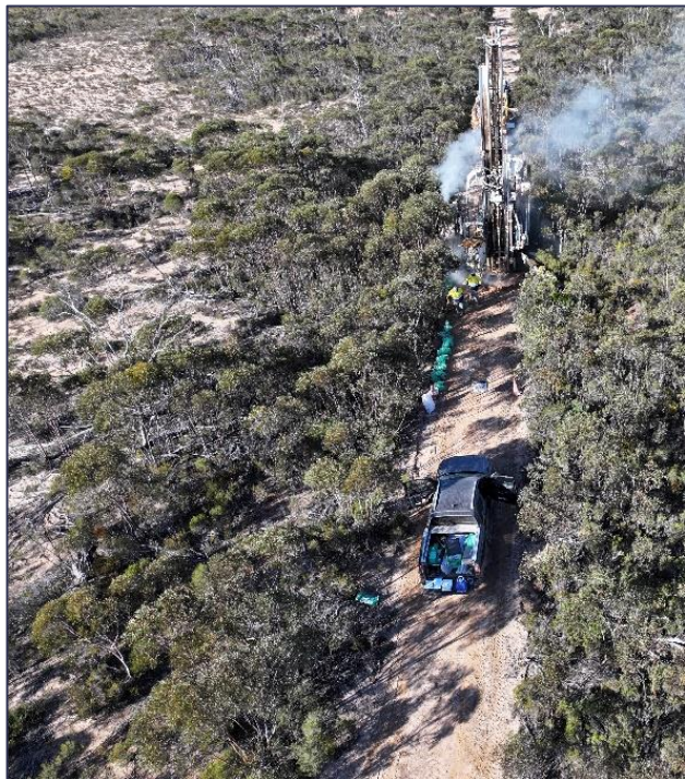
Above: Air core drilling south of the Newmont deposit, May 2024.
