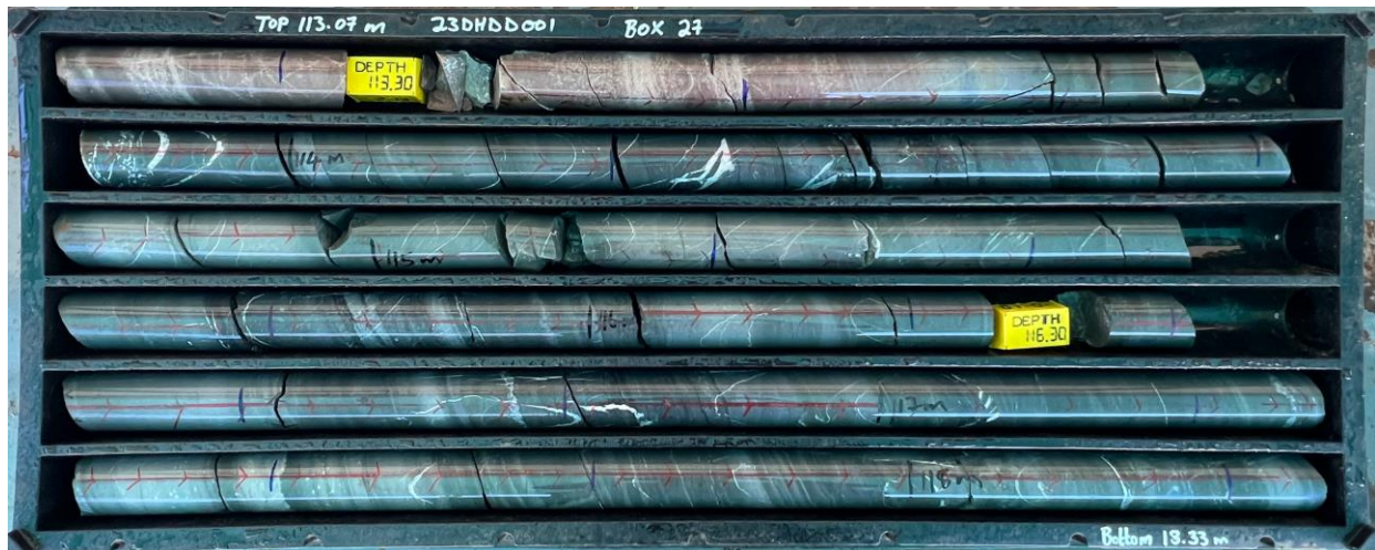
Figure 4. Drill core from 23DHDD001 showing bedded siltstone units with brittle fractures and Quartz-Carbonate veining with chalcopyrite and chalcocite mineralisation from 113-118m.
