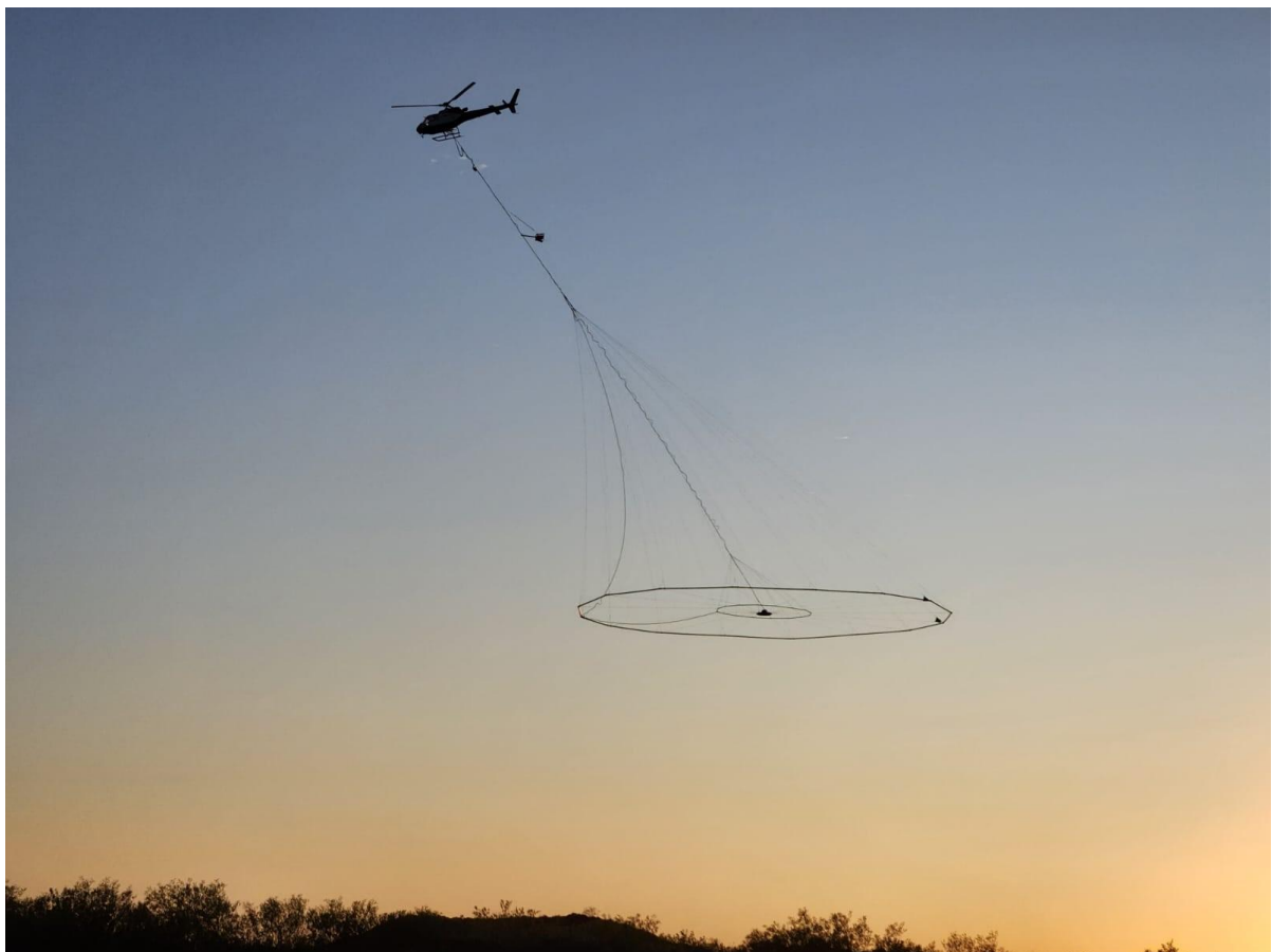
Figure 1 – VTEM being flown over Oonagalabi project location.
