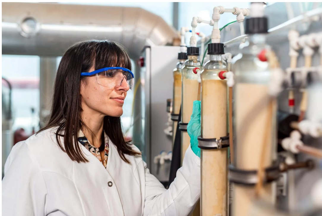
Figure 1 – Laboratory testing apparatus Containing Vulcan's Proprietary VULSORB® Sorbent 1 . VULSORB® sorbent, a next-generation material engineered to enhance lithium recovery in magnesium-rich brines and minimise water consumption, a key factor for sustainable lithium extraction in Bolivia's salars.
