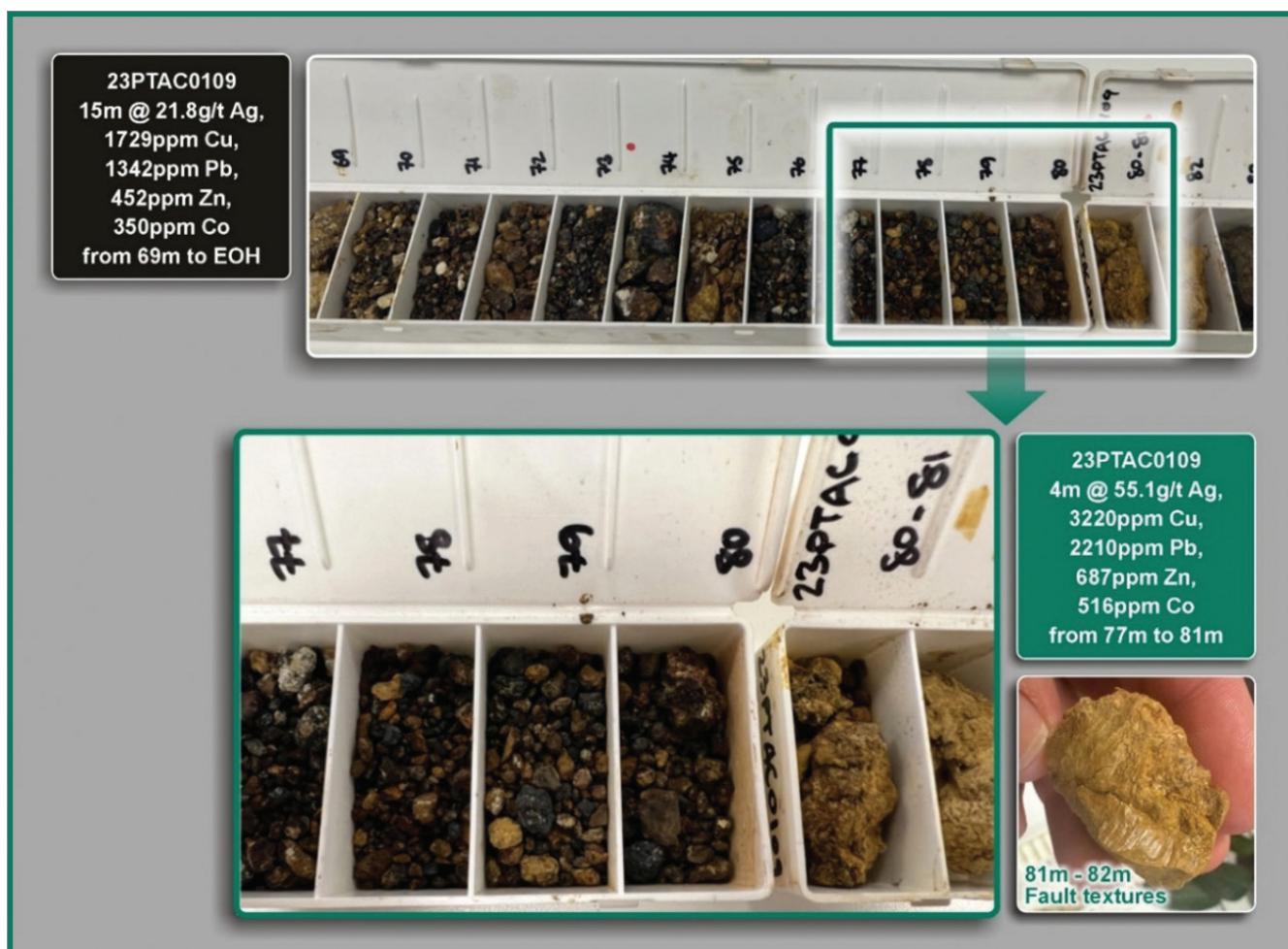
Photo 1 - Gossanous samples in chip trays from Haddon drillhole 23PTAC0109 (assays reported in release dated 5 March 2024)
