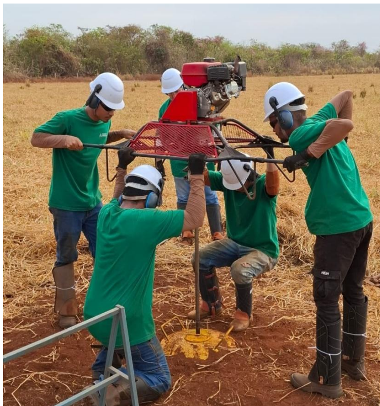
Figure 2. Auger drilling at Santa Anna Project 19 January 2026.
