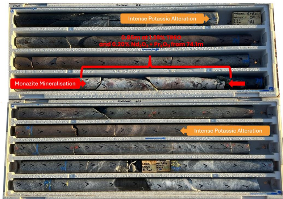
Figure 2: MWDD001 structurally controlled carbonatite dyke, 0.85m at 1.39% TREO and 0.20% \text{Nd}_2\text{O}_3 + \text{Pr}_6\text{O}_{11} from 74.1m within intense potassic alteration halo. The mineralisation represents a new REE mineralisation lode not observed at surface.
