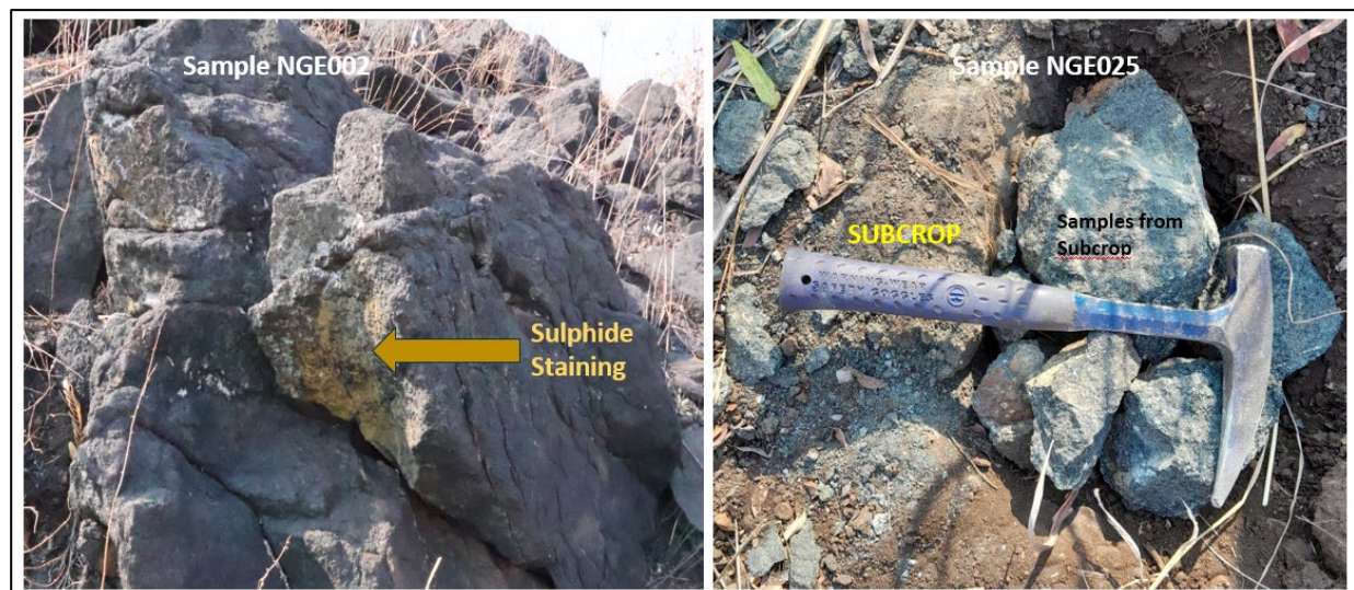
Figure 2: Sulphide staining and chrysocolla mineralisation in samples NGE002 & NGE025
