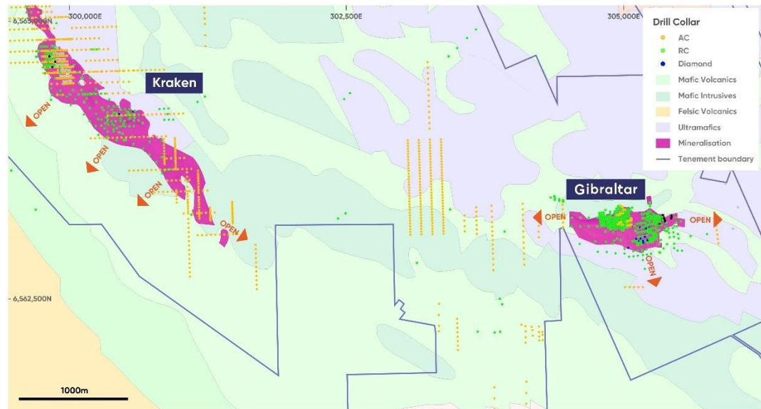
Figure 18 – Kraken - Gibraltar prospect trend with interpreted mineralisation and drill hole coverage
