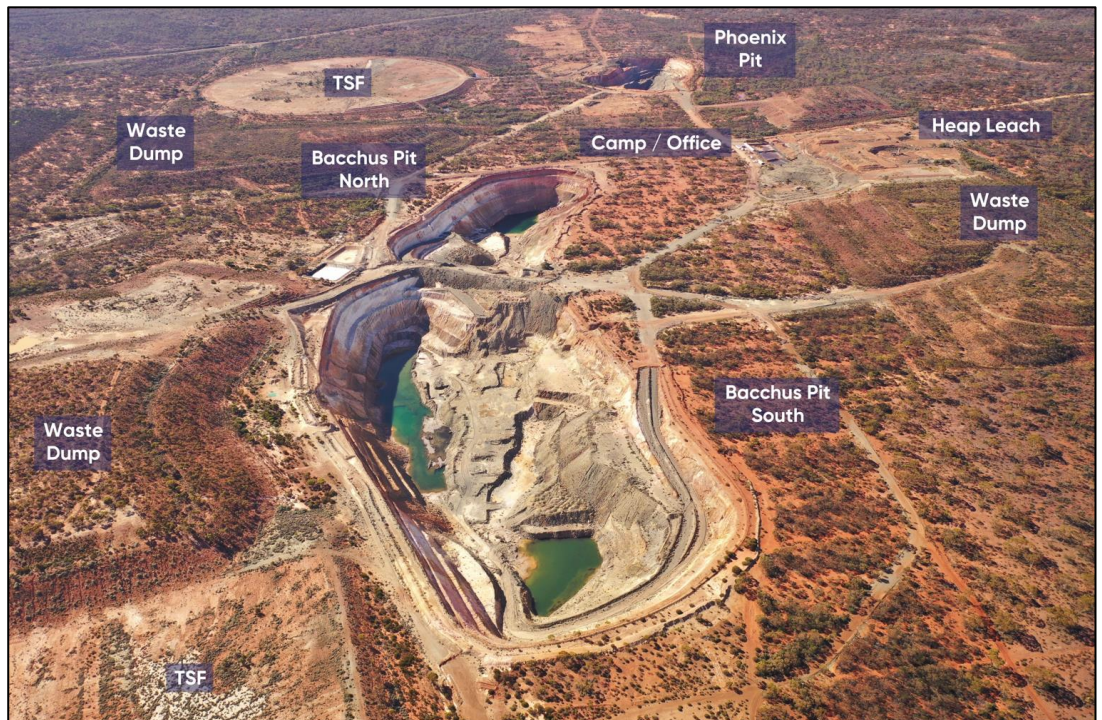
Figure 4 – Image looking north showing former Bullabulling open pits and surface infrastructure
