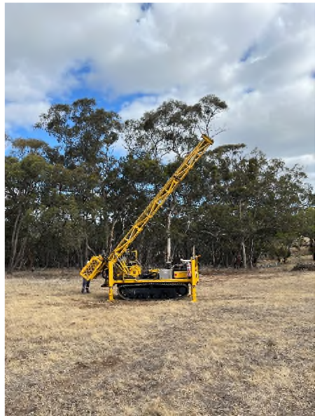
Figure 2– Irvine Project (Stawell zone) – Diamond drill rig mobilised to site
