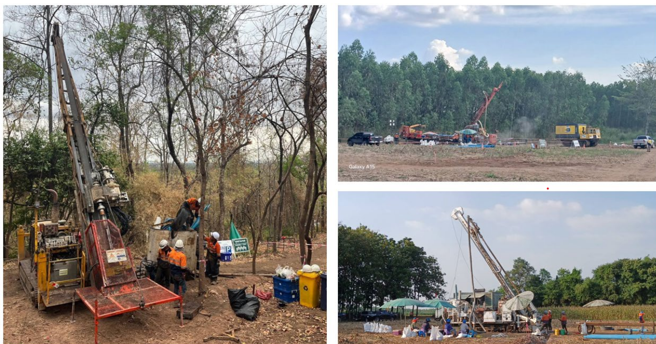
Figure 2: Reverse Circulation (“RC”) and Diamond Drill (“DD”) rigs drilling at Chatree SE Complex.
