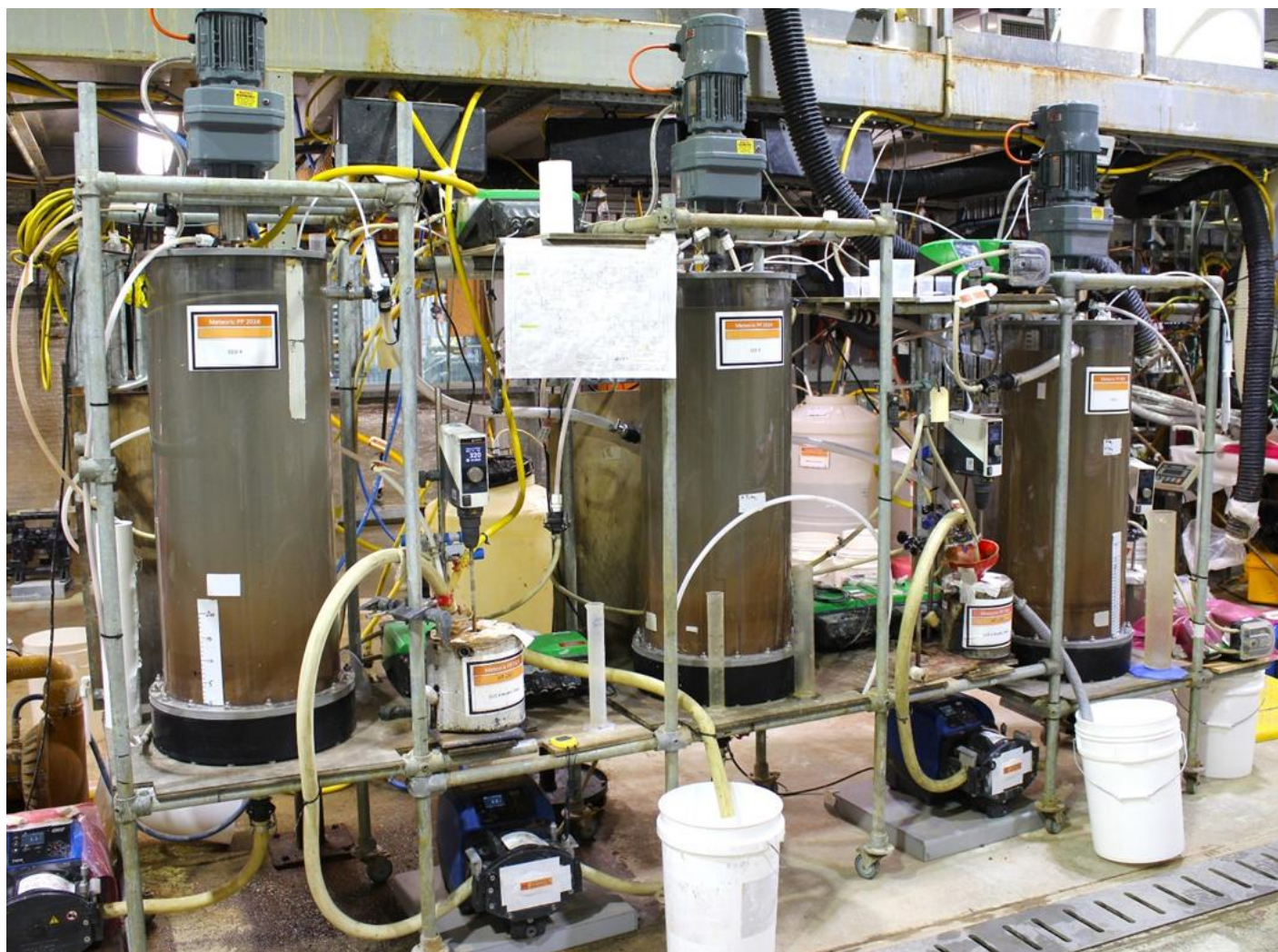
Figure 2: Counter Current Decantation (CCD) Wash circuit
