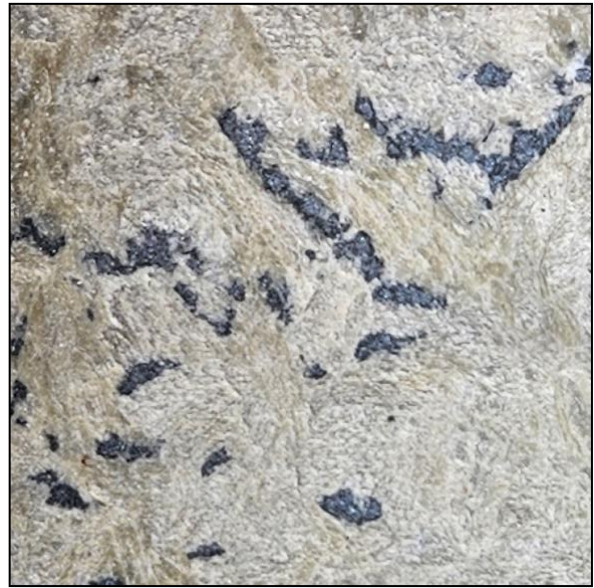
Figure 2: Coarsely disseminated tetrahedrite (copper – antimony sulphide) in massive siderite and barite veining. Drill core from BPD08.
