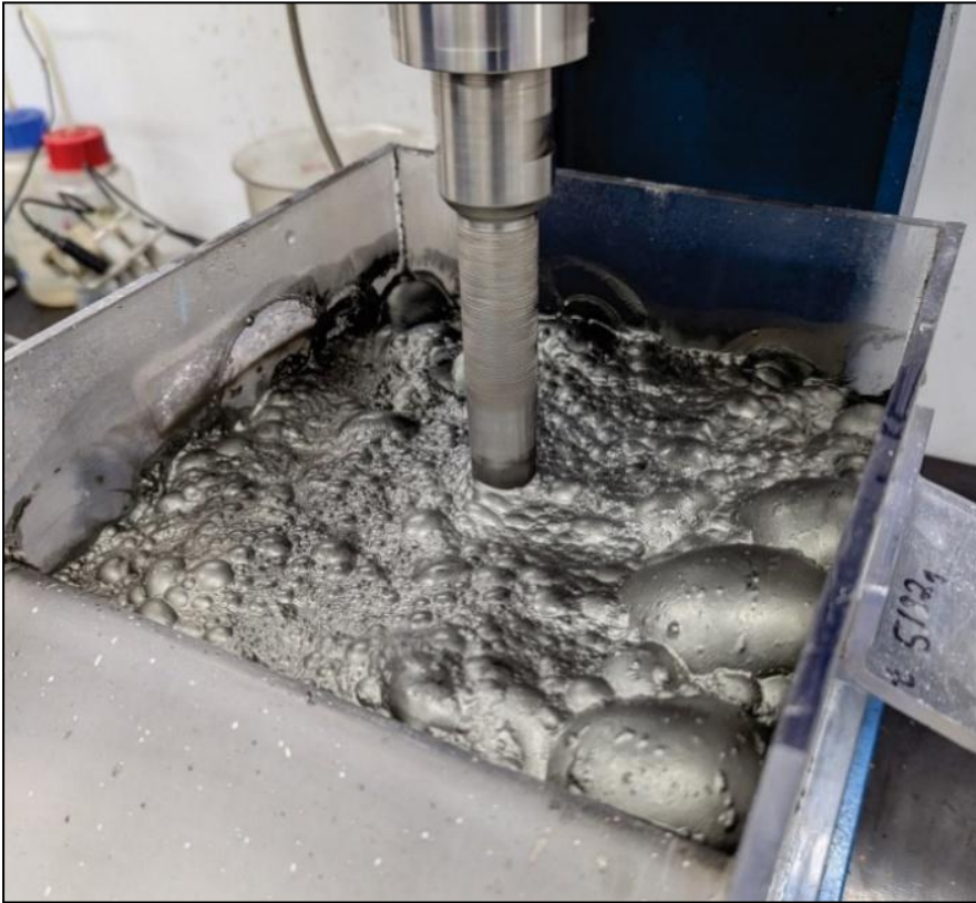
Figure 6: Copper-antimony-silver concentrate from Bulla Park, first flotation test run, at Core Resources Pty Ltd
