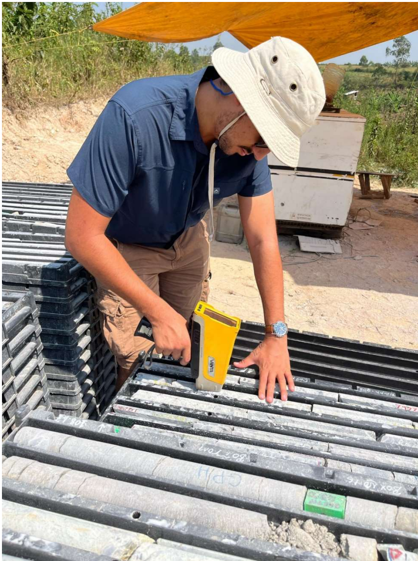
Figure 2: Field activities with XRF analyser
