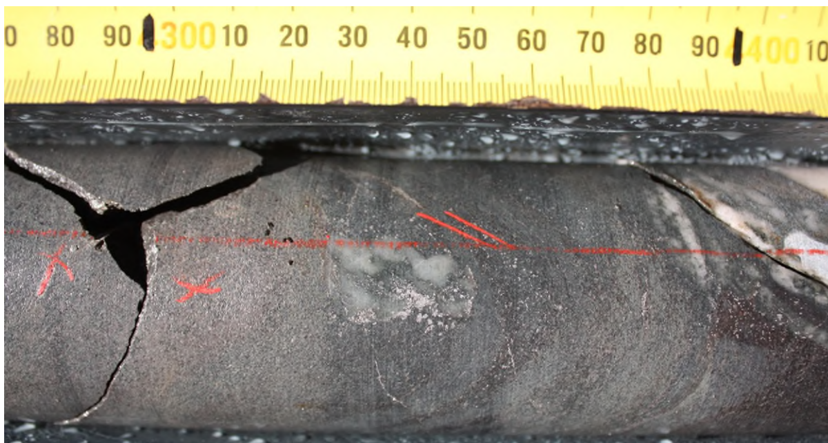
Figure 6. RD045 406.2 – 406.3. fine grained arsenopyrite intergrowth around silica within disseminated pyrrhotite groundmass.
