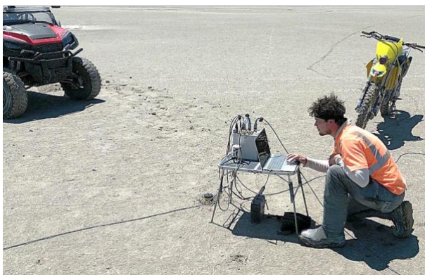
Figures 3, 4 and 5 : Lithium Energy geophysical team members conducting MT survey at White Plains Project, Utah, USA
