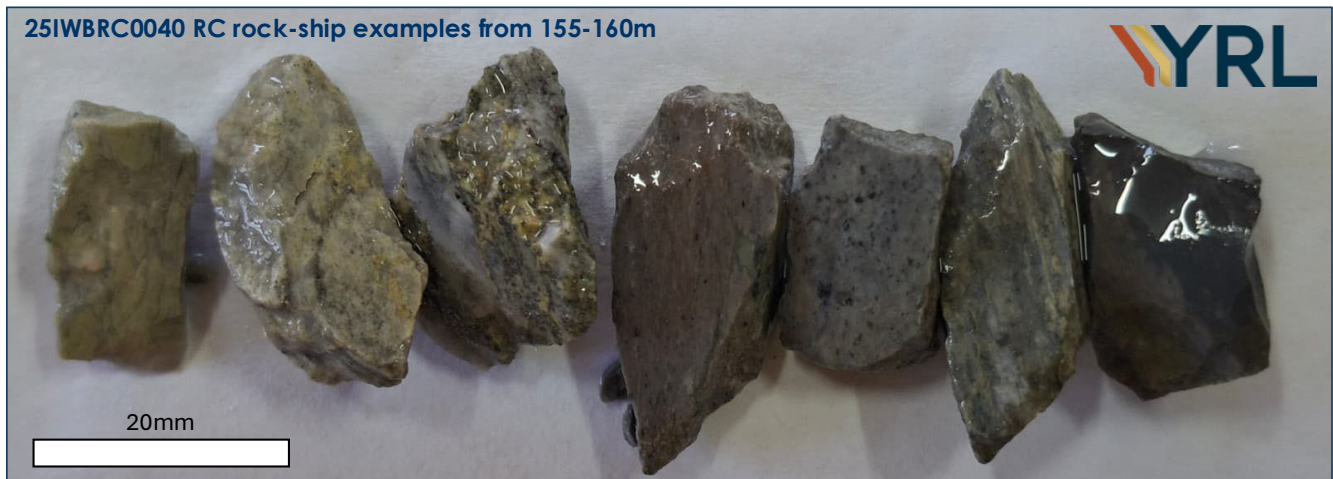
Figure 3: Example of rock chips obtained from 25IWBRC0040 between 155m and 160m downhole. RC chips from this interval display intense alteration, including silica-albite-carbonate alteration (+/- biotite, chlorite and sericite) with disseminated fine to medium-grained pyrite and arsenopyrite up to 5% within some chips, or as stringers parallel to fine veins or the dominant foliation.
